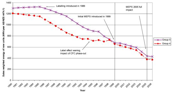
Figure 4: Energy Consumption Trends in Australia – New Refrigerator-Freezers
