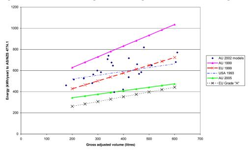
Figure 2: International Comparison - Group 4: Manual Defrost Refrigerator-Freezers
